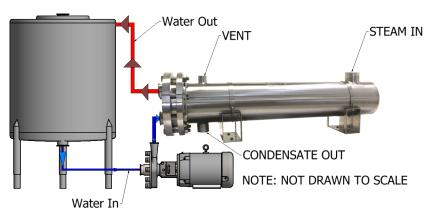
Standard hot liquor heat exchanger setup
